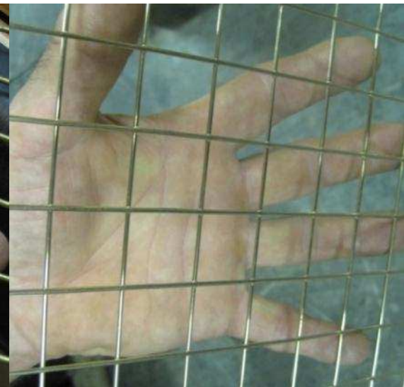
Seawire™ welded mesh, 1.5mm welded Cu-Si Seawire点焊网，1.5毫米铜硅合金焊接
